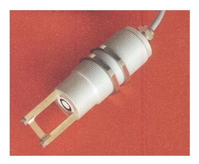
The sensor U 2000 is an ultrasonic distance sensor with integrated electronics for processing precise measurements on virtually all materials. The sensor is equipped with an RS232-interface Data output and configuration features. Thanks to the external trigger input can be connected to a second sensor. A thickness measurement system set up with time synchronized measurements.
